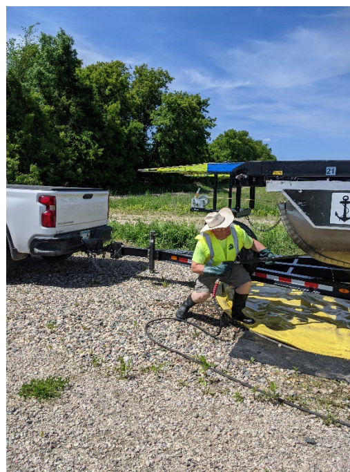
Figure 8. A level 2 inspector decontaminating a barge with high pressure
